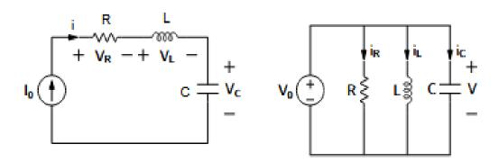
\* A series RLC circuit driven by a constant current source is trivial to analyze. Since the current through each element is known, the voltage can be found in a straightforward manner.
